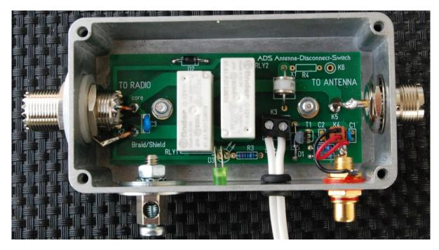
Note: The SO259 bulkhead socket "TO ANTENNA" and the RCA Phono Plug "REMOTE OFF" must be mounted completely isolated against the metal box. For this purpose a specific set of isolation washer and busher is needed.
