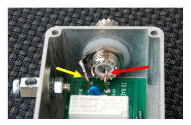
wire from K1 in the opening of the rf-bulkhead socket's core conductor. Fill the hole with solder. Hint: Screw a PL259 Plug at the outside to avoid deformation of the socket's insulation caused by the soldering heat.
